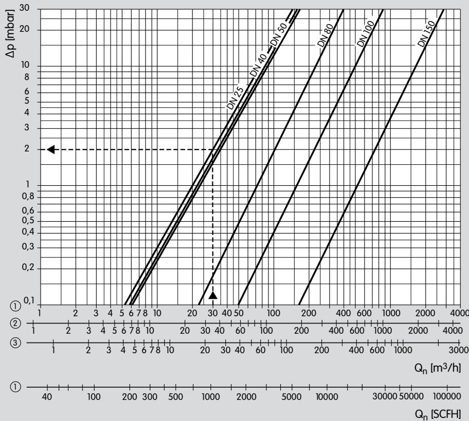
When reading off the values, operating cubic metres must be used. Then the pressure loss  $\Delta p$  read must be multiplied by the absolute inlet pressure  $p_u$  in bar (positive pressure + 1) to account for the change in the medium's density.
