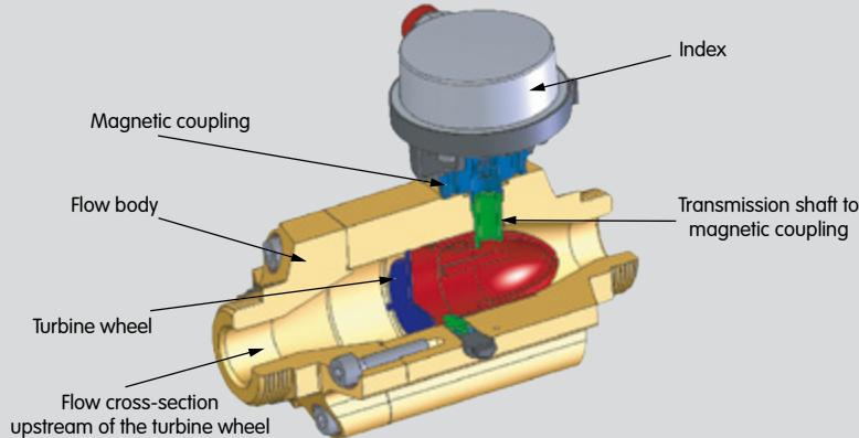
Flow meters DM and DE are identical as regards their flow behaviour and basic design. The flow volume drives a turbine wheel. A magnetic coupling is used to transfer the rotary movement of the turbine wheel to the index. The rotational speed of the turbine wheel is proportional to the flow rate of the medium flowing through the meter.
