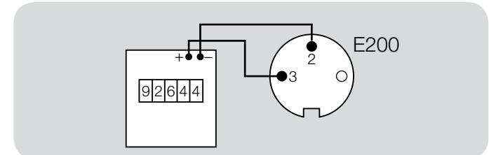
Electronic meter for digital remote indication of the current flow rate (in m<sup>3</sup>/h).
