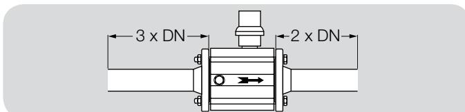
The pipe downstream of the flow meter must not have any restriction point which could cause the flow to back up. All approved flat seal types may be used.
