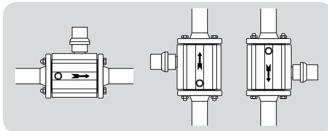
Flow meters in the threaded version and with an E200 pulse output can be used for flow control. For this application, the DM/DE..R must be installed in the horizontal position with the index facing upwards.
