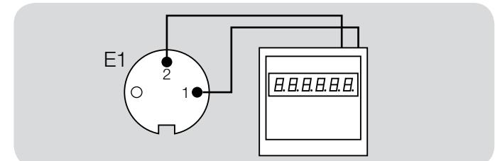
Electronic meter for digital remote indication of the total flow rate (in m<sup>3</sup>).
