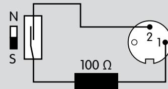
Max. switching voltage:  $U_{max} = 24$  V,
