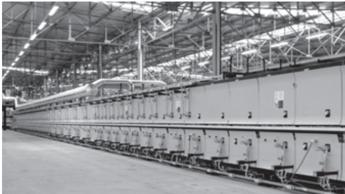
Ceramics industry: roller hearth kiln
