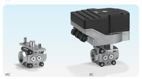
The IFC is composed of linear flow control VFC and actuator IC 20 or IC 40. It is designed to adjust volumes of gas and cold air on various appliances. The IFC is designed for control ratios up to 25:1 and is suitable for regulating flow rates for modulating or stage-controlled combustion processes.
