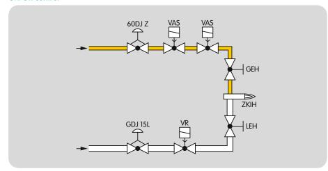
The gas/air mixture is set using the gas adjusting cock GEH and the air adjusting cock LEH. For a constant mixture of gas and air (lambda), one pressure regulator per burner is used in the gas and air circuits.
