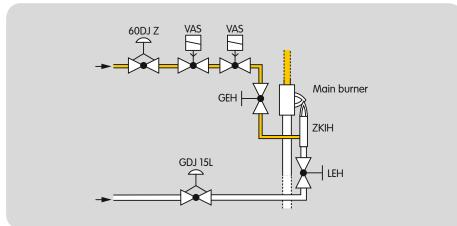
Install the pilot burner so that reliable ignition of the main burner is guaranteed.
